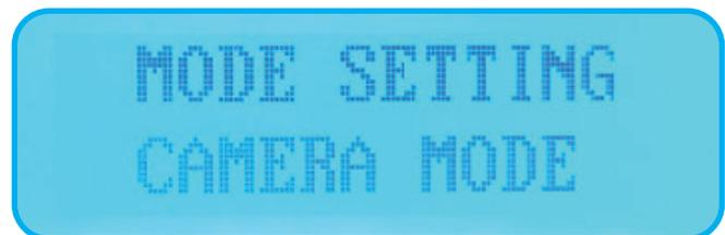
1. Press ENTER to highlight the mode selection (text will change to blue). Use the DOWN button to toggle between "Fixed Length" and "Camera Mode." Press ENTER to confirm your selection.
