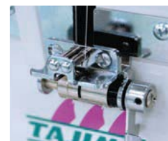
Middle thread guide with thread take-up spring
