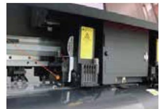
Equipped with a media jam sensor, the risk of print head failure is reduced even in situations where jams occur. This greatly reduces the risk of failure due to media jams on glue surfaces in the unlikely event of a media jam.
