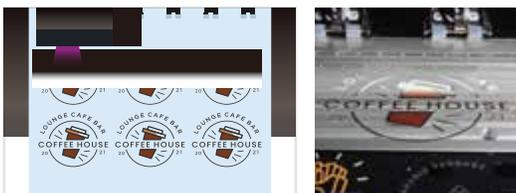
Designs are printed on special glued film, then application sheet is pasted on the film automatically.
